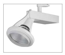
Spotlight for ceramic metal halide 150W G12. Die cast aluminium body, powder coat painted. Integral electronic control gear. Rotation 355°. Vertical adjustment +/- 90°. Track mounted with 3-circuit adapter. Voltage 230V. Light source to be ordered separately.
